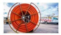
Roll of conduit - used to enclose coax and fiber-optic cable underground
