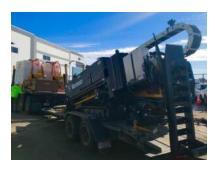
Directional Drill – used to create an underground path for the network
