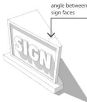
Figure 7.6(3)(d)(2) Measurement of Sign Area, Double-Faced Signs
