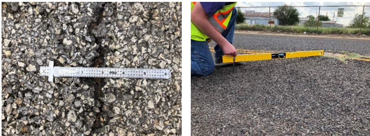
Figure 5. Typical PCI Field Measurements
