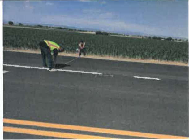
Image 10 – Lane widths along WCR 5 do not measure to be 12-foot wide. Striping widths do not measure to be 8-inches wide.
